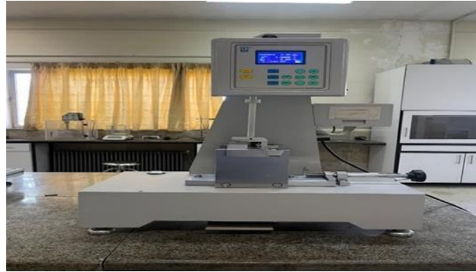
Figure 4. The impact testing machine made by Gutec Model (GT-70-45MDN)
