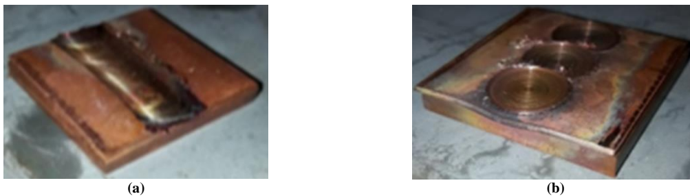
Figure 2. Tool advancement methods in copper thin sheet welding process. (a) horizontal advance, (b) vertical advance.
