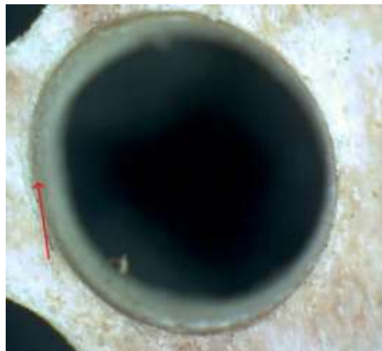
Figure 4. Drilling with 34.32 N force
