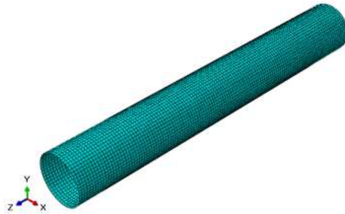
Figure 1 A view of the elements made for the shaft in Abaqus software
