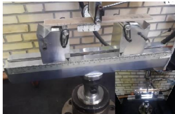
Figure 2. Composite part during three-point bending test.
