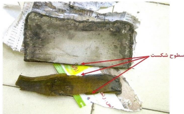
Figure 2 A view of the fracture surface of the studied sample
