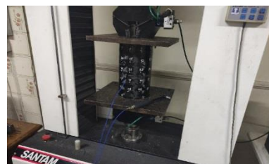
Figure 6. Sample configuration for vibration correlation test
