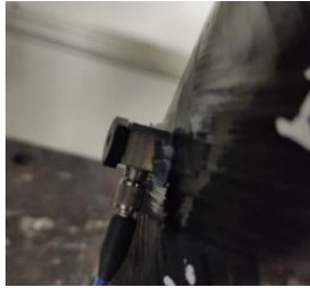
Figure 4. Connecting the accelerometer to the sample
