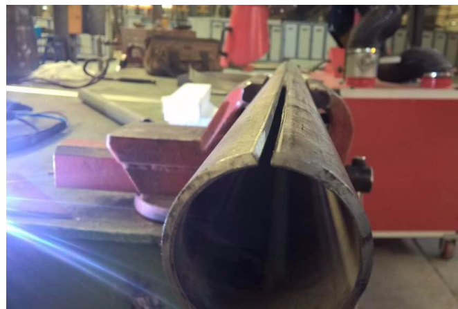
Figure 2. The sample type with a 60 degree chamfer
