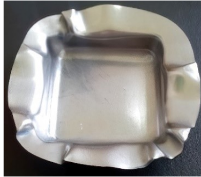
Figure 4. Steel sample formed with rubber matrix die and intermediate ring
