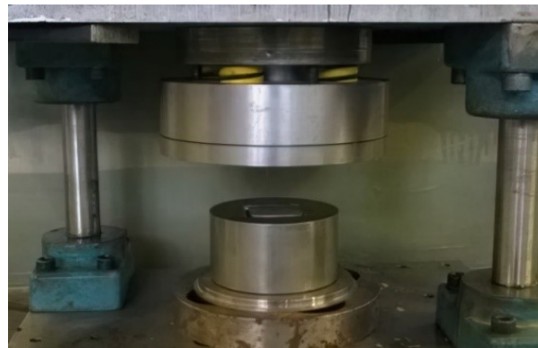
Figure 2. The fabricated die with the metal die.
