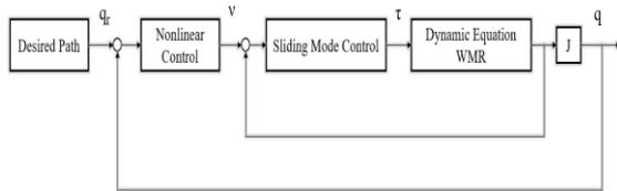
Fig 2. Block diagram of a non-linear control system
