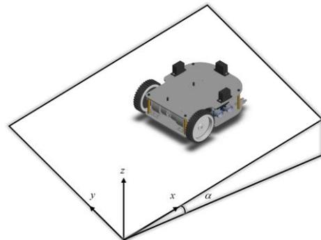
Fig 1. The nonholonomic mobile robot on the slope
